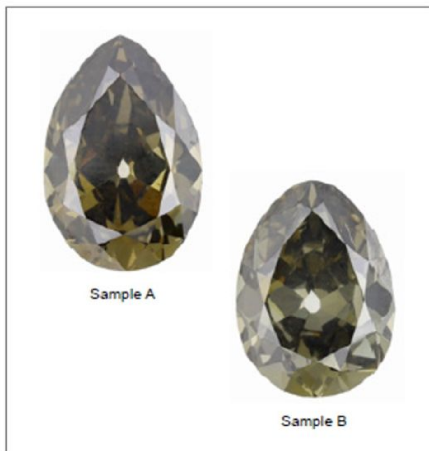
Figure 2: The two pear-shaped old-cut diamonds were unmounted from the brooch in Figure 1 for further examination. Sample A measures 16.07 \times 10.81 \times 6.58 mm and has a dark greenish brownish grey colour; sample B is 14.18 \times 10.43 \times 5.89 mm and is dark greenish grey. They are both type IIb diamonds. Composite photo by A. Delaunay, © LFG.
